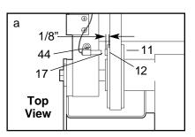
Screw (44) and move the Reed Switch slightly. Retighten the Screw. Re-attach the hood and run the treadmill for a few minutes to check for a correct speed reading.
